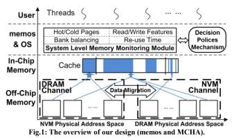
main memory utilization vertically when mapping pages. Finally, for a specific sub-memory system, DPM employs the proper memory policies (partitioning and rebalancing) based on the characteristics of incoming memory requests.
