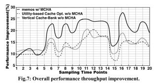
accessed pages from all channels are allocated to use a larger amount of LLC, and channel-level bandwidth utilization are nearly balanced. Moreover, memos improves QoS (indicated by Max Slowdown) [6,8,11] significantly (23.6% on average).
